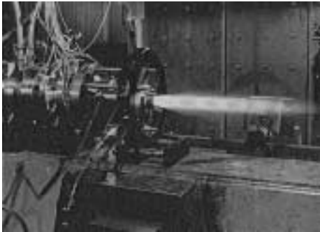
Figure 3. SFRJ combustor performance testing.
