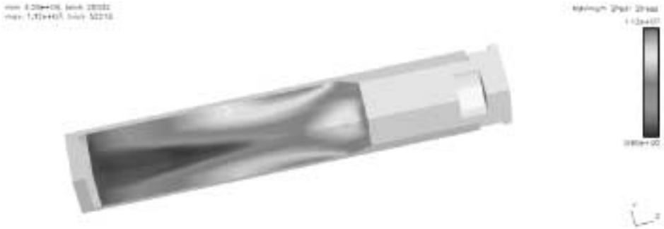
Figure 5 – Maximum stress state with the chamfer including a friction coefficient of 0.05 between the explosive and case.
