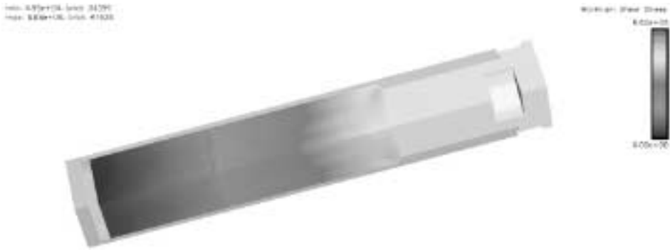
Figure 3 – Maximum stress state without friction between the explosive and case.
