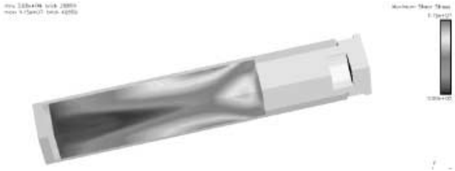
Figure 4 – Maximum stress state with friction coefficient of 0.05 between the explosive and case.
