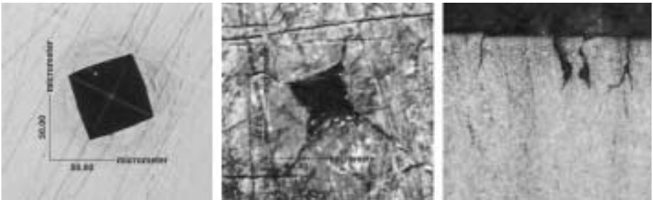
Fig. 4. Surface and cross sectional images of the barrel material (FFZ).
