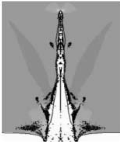
Figure 4 – Comparison of hydrocode with experiment (solid line) for shaped charge in sand.
