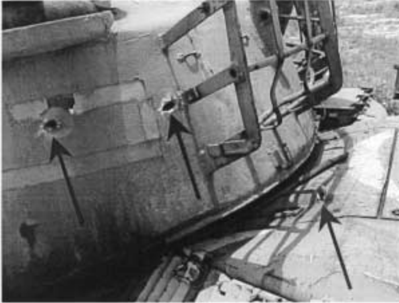
Figure 4. 30 mm APFSDS-T full penetrations into a M-60 tank-turret @ 1500 m.
