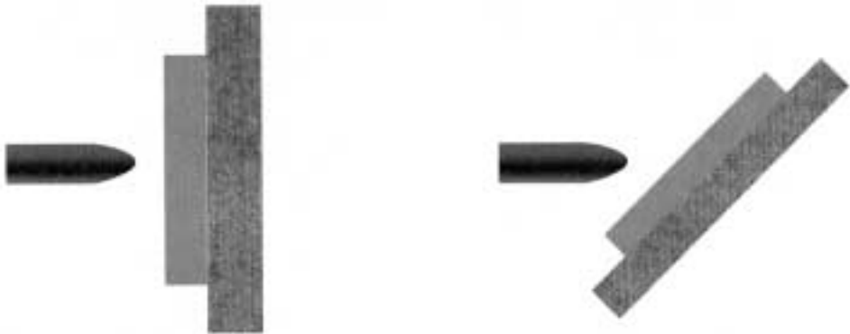
Figure 2. Schematic of experimental arrangement, line-of-fire thickness held constant.
