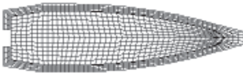
Figure 1: Mesh description of the 7.62 mm NATO Ball round.
