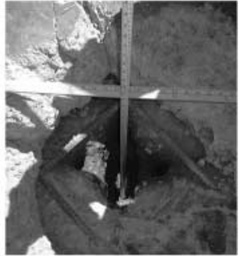
Figure 1d. Target damage from 4 + 1 charge.
