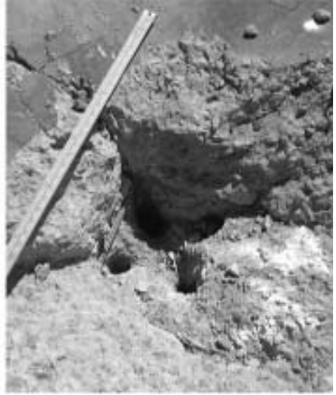
Figure 1b. Target damage from 4 charges.
