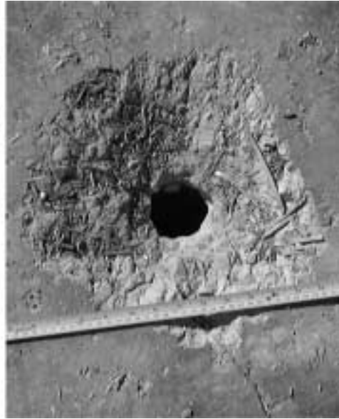
Figure 2b. Target damage from 1 charge.
