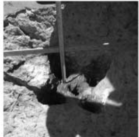
Figure 2d. Target damage from 1+4 charges.
