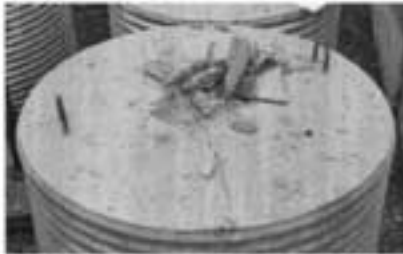
Figure 8. Effects of standoff on performance. (Clockwise – 1/2, 1 and 2 charge diameters)
