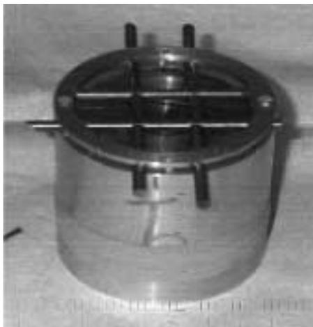
Figure 4: Subscale test warhead.
