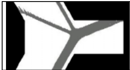
Fig. 6: The resulting outflow in the simulation with S=5 and initial 1,09 mm gap between the lower incoming flow and the collision plane.
